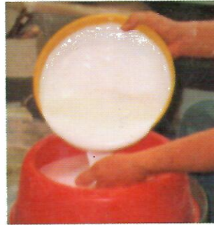
Make plaster bats
